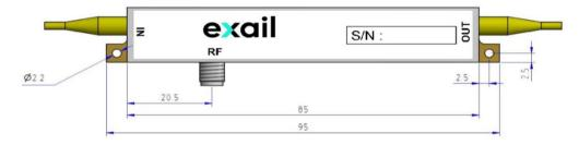
Thickness : 9.6mm Material : KOVAR Package dimensions in mm
