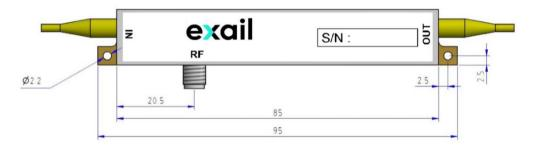
Thickness: 9.6mm Material: KOVAR Package dimensions in mm
