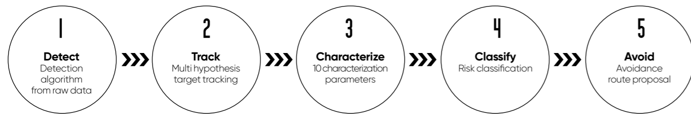
SeapiX-FLS detection process
