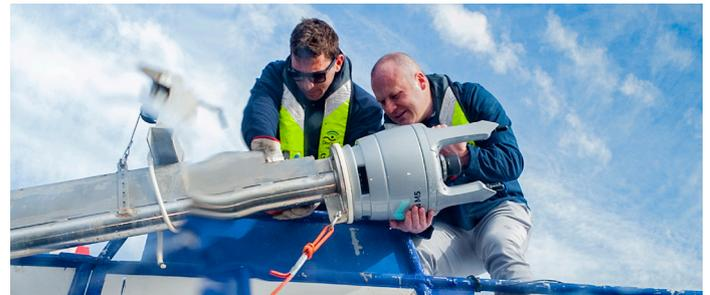
Compact, lightweight, and pre-calibrated, Gaps systems can be quickly deployed from over-the-side poles, stingers and confined spaces
