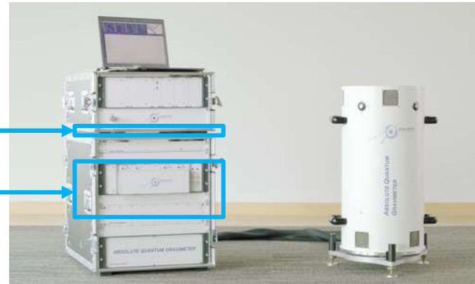
Light-pulse atom interferometry using cold Rb atoms
