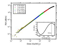
Image from D. D. Francesca et al., "Qualification and Calibration of Single-Mode Phosphosilicate Optical Fiber for Dosimetry at CERN," in Journal of Lightwave Technology, vol. 37, no. 18, pp. 4643-4649, 15 Sept. 15, 2019, doi: 10.1109/ JLT.2019.2915510
