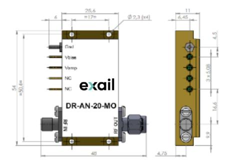
The heat-sinking of the module is necessary. It's user responsability to use an adequate heat-sink. Refer to page 5 for Exail recommended heat-sink.
