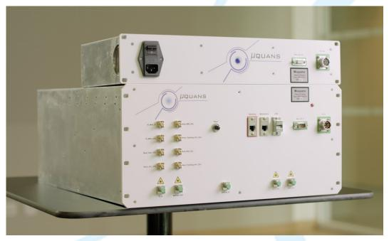
This unique industry-grade regeneration laser station has been developed in collaboration with LPL (Univ. Paris 13) and LNE-SYRTE (Observatoire de Paris) laboratories, in the frame of the REFIMEVE+ project
