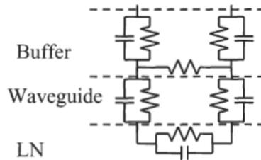
*Figure 9: Equivalent RC circuit model of the MZM crystal electric structure, with vertical and horizontal components.*
