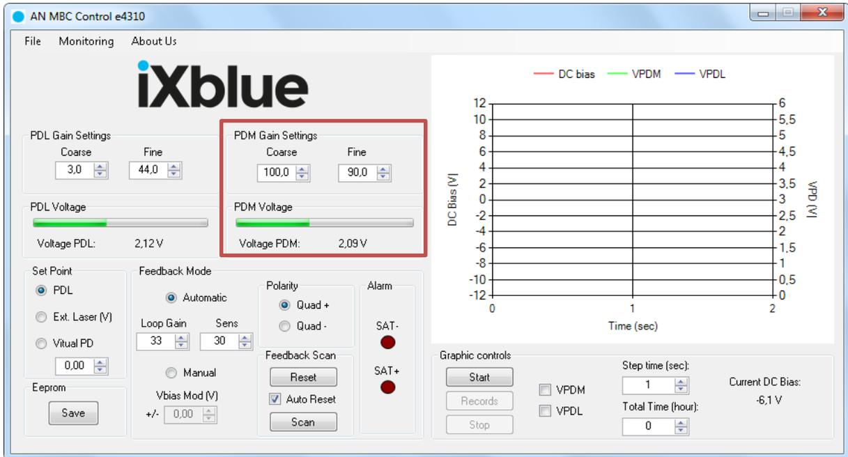
Figure 3: PDM adjustment
