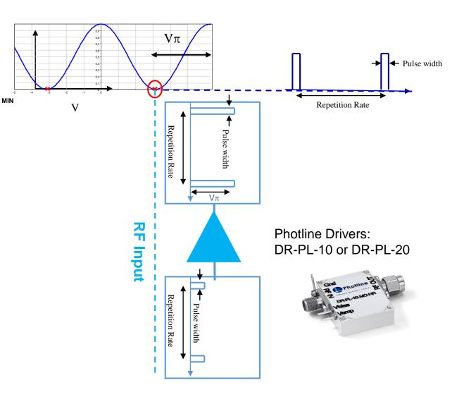
\*FRR = Frequency Repetition Rate \*\*PW: Pulse Width
