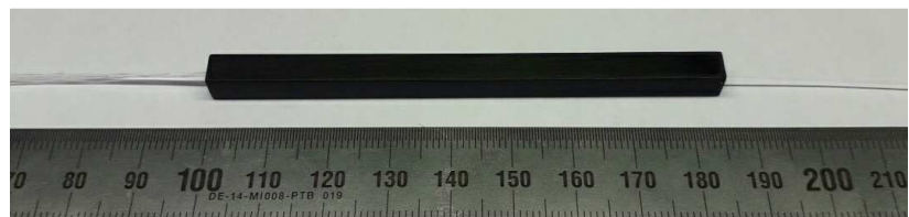
Fig 4. Packaging of the combiner/fan-in spliced to the 12c-EYDF
