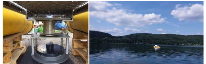
Figure 1: (left) Echoes 10 000 implemented on the USV cataraft; (right) remotely controlled cataraft on Lake Laacher See during the field campaign in 2019
