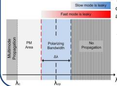
Transmission spectra showing two separate cut-offs for the polarization modes in the fast and slow axes at different spectral positions.
