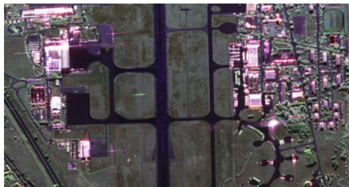
20cm resolution X band SAR image, Courtesy of ONERA
